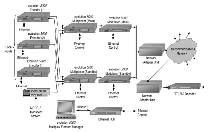
Figure 1.6: Typical Compression System
